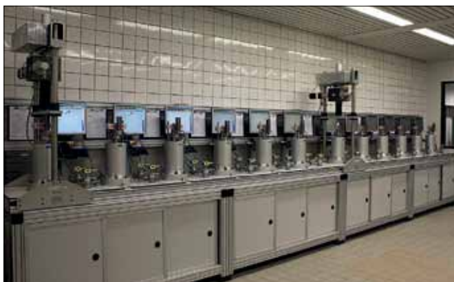
Fig. 7: Triaxial test bench of the Geomechanical Test Lab, RWE Power AG, Bergheim
