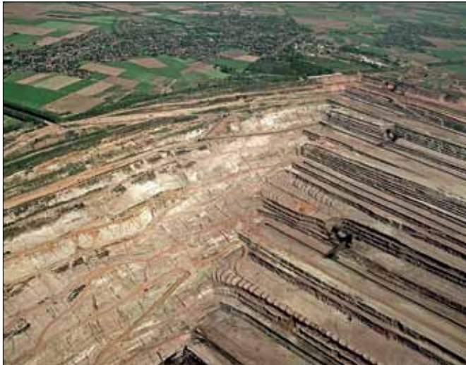
Fig. 10: Operation of narrow berms along the mine-rim slope, taking the Hambach mine as example
