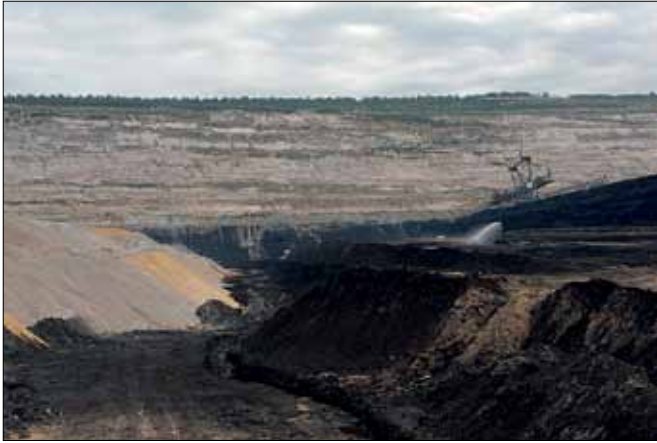
Fig. 5: Hambach mine: dumping follows extraction directly in the mine floor
