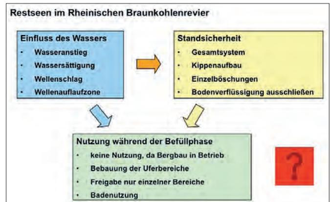
Fig. 4: Water – a factor influencing stability that needs to be examined with a view to use perspectives
